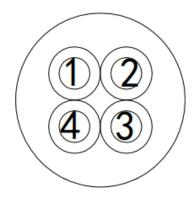
Cable Marking: RS PRO 4 Core×0.34mm<sup>2</sup> Unscreened Industrial Cable 250V
