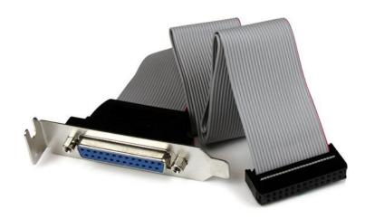
The PLATE25F16LP DB25 to IDC26 Parallel Port Bracket adds a DB25 parallel port to the rear panel of a low profile/small form factor computer, which connects to an IDC26 header connector on the motherboard.
