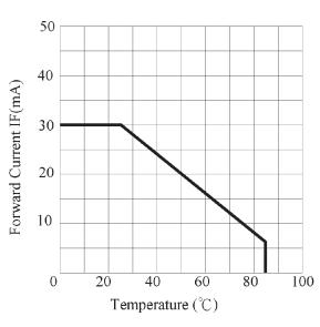
FORWARD CURRENT VS. AMBIENT TEMPERATURE
