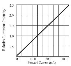
FORWARD CURRENT VS. LUMINOUS INTENSITY
