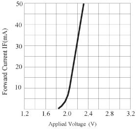
FORWARD CURRENT VS.APPLIED VOLTAGE
