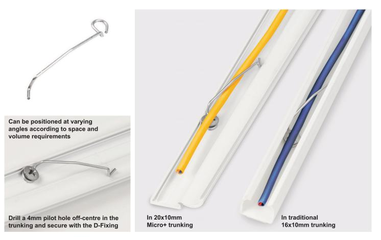
Safe-D Spring Clips effectively secure single cables (<7mm o/d), either direct to surface or in PVC micro trunkings.
