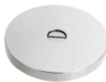
To achieve the optimum pull force 100% contact area must be achieved using the recommended armature plate. The force will be affected if other material specifications, thicknesses and surfaces are used, or if the armature fails to make positive contact over the full diameter of the face of the magnet. Where misalignment is likely to be an issue we recommend that an oversized armature plate is used to ensure 100% full contact, this however will reduce the stated pull force by approximately 10%.
