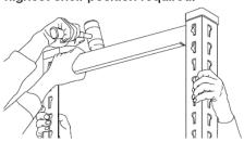
To locate beams: Clip lugs at the ends of the beam into the 'P' slots in the upright. Press down, then tap into place ensuring lugs are fully located to the base of the slots.
