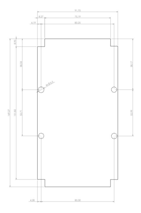
Dashed line shows outline of the mounting boss under PCB board Recommended mounting holes diameter Ø3,5mm
