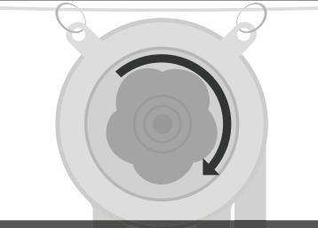
5. You can adjust the tensile level of the balancer by turning the rotator before use to avoid elastic fatigue which is caused by overload.
