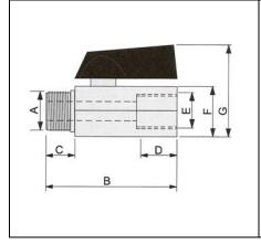
Suitable for domestic water services, heating, air conditioning plants and compressed air systems Minimum Working Temperature: 0°C Maximum Working Temperature: 90°C Valve body manufactured from brass with a bright chrome finish
