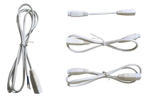
The RS Pro CCT Link Light range has a number of link lead accessories and power lead that can be purchased separately. Power lead is available at a length of 1.8m allowing plenty of flex on installation. Link leads come in lengths of 150/500/1000mm depending on the needs of the user.
