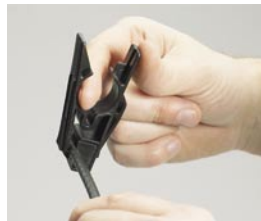
Insert cable, rotate and pull of scrap
