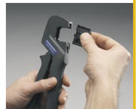
Quick fit/release of crimp dies
