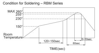
The condition mentioned above is the temperature on the Cu foil of the PCB surface. There are cases where board's temperature greatly differs from switch's surface temperature depending on board's material, size, thickness, etc. Care, therefore, should be used not to allow switch's surface temperature to exceed 260°C.
