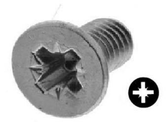
Countersunk, also known as flat head machine screws, are designed for ease of assembly and these particular machine screws with their cross recess drives are a popular driving method with this type of fastener, as they allow the head to sink into the material. Machine screws can be used in pre-tapped holes or used with conforming nuts and washers in through holes.
