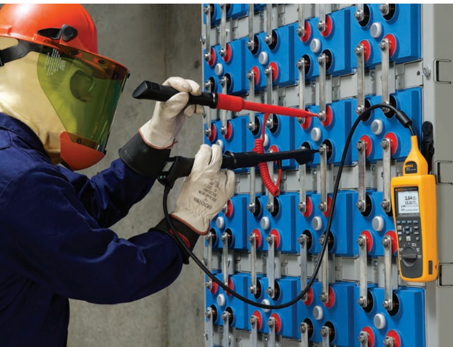
Measuring ohmic values in sequence mode
