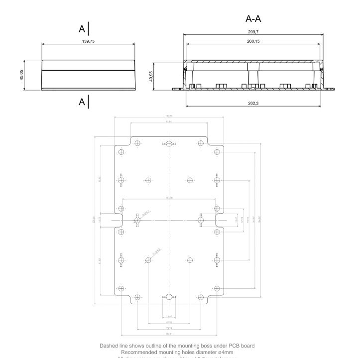
All dimensions are given within +/-0,5mm tolerance
