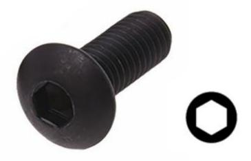
Button Head Socket Screws are designed for light duty. They have a similar thread design as a Socket Cap Screw although the dome-shaped head is wider and has a lower profile than a Socket Cap Screw, presenting an aesthetic appearance in an assembly. These fasteners are ideal when a wider bearing surface is required.
