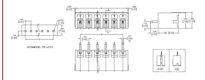
Positions: 02 thru 24 A= .150 [3.81] x No. of Spaces + .181 [4.60] B= .150 [3.81] x No. of Spaces
