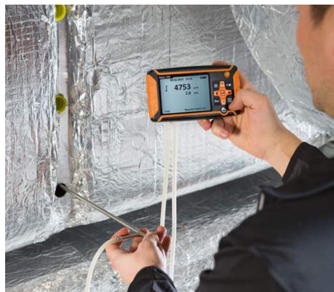
Removable instrument allows Pitot tube measurements in ducts (Pitot tube available separately)
