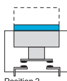
Operating principle of an enabling switch
