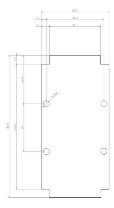
Dashed line shows outline of the mounting boss under PCB board Recommended mounting holes diameter ø3,5mm
