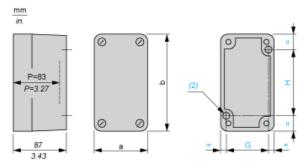
(2) 2 x Ø 5.6 mm/4.94 in. holes, depth 12 mm/0.47 in. P Usable depth
