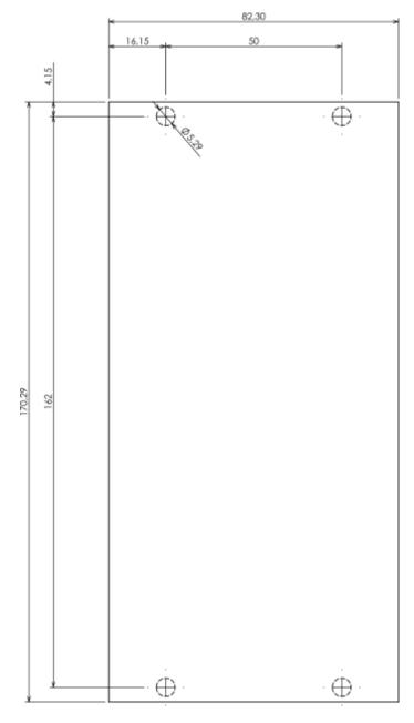
Dashed line shows outline of the mounting boss under PCB board Recommended mounting holes diameter ø3.5 mm
