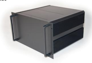
The HS-19 Series of rack mounted 19" heatsink enclosures is a versatile and user friendly 19" enclosure series. Designed for both professional users and home hobbyists alike, HS-19 features extruded aluminum heatsink side panels. The high grade aluminum body features removable top and bottom panels providing easy access to work inside.
