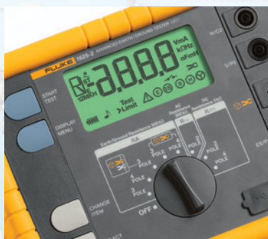
Use the Fluke 1625-2 to determine the health of your earth ground systems.
