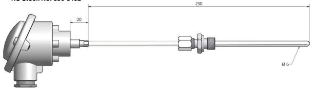
Thermocouple J. Ø6 x 250. Sliding fitting
