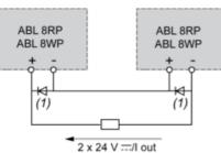
(1) Two Shottky diodes Imin = power supply In and Vmin = 50 V  $\,$
