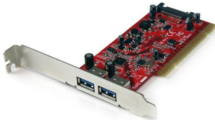
The PCIUSB3S22 2-Port PCI to USB 3.0 Card enables you to connect USB 3.0 peripherals to a PC through a legacy PCI host bus, which doubles the data transfer speeds when used with USB 3.0 peripherals than would be possible with a USB 2.0 host connection - up to 1.3 Gbps (PCI bus limit).
