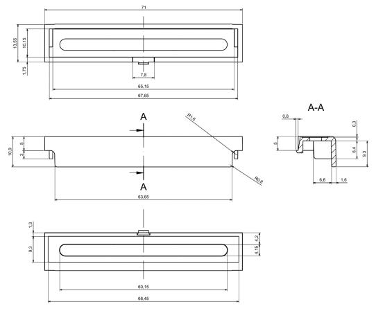
All dimensions are given within +/-0,5mm tolerance
