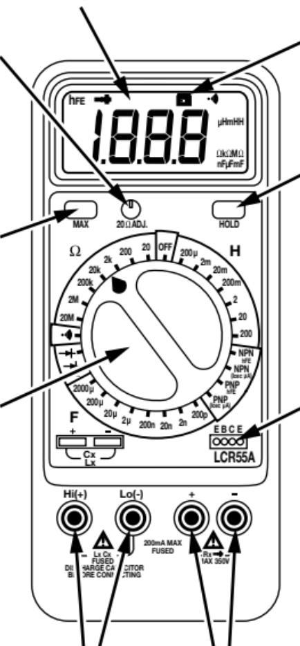
High (+) and Low (-) inputs for capacitance
