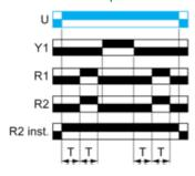
Function Di: Symmetrical Flashing Relay (Starting Pulse On)
