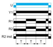
Function Dt: Symmetrical Flashing Relay (Starting Pulse Off) & With Pause / Summation Control
