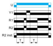
Function C: Off-Delay Relay with Control Signal
