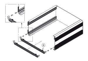
2. Install (6) GP Bar Kit [option] into the slide rail slot in side frame and secure with GP Bar position by Umbrella Phillips Screw M5-10 (Dog Point). We advise to install user components at this stage. Our GP Bar Kits are ideal for this purpose, but user can prepare their own method.
