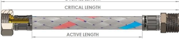
Critical length is the distance between hose mating faces. This must be 10% greater than the actual distance between the two corresponding fixed mating parts to avoid tensile stress whilst in service.
