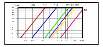
Schedule 2: Pressure loss for type of end connection based in internal diameter (DN) Formulae:  $P2 = P3 \times R$
