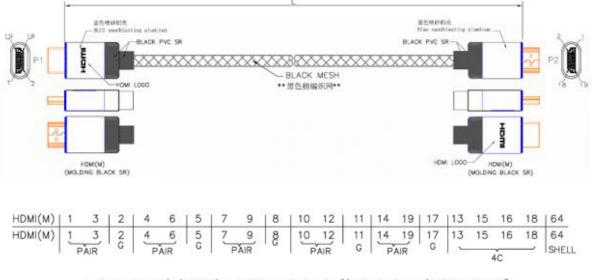
CABLE: 28AWG(1/0.32BC),UL20276,AL+B+D-FOIL,[(#28\*1P+D+FAM)\*5PCS+#28\*4C], BLACK COLOR,OD=7.3±0.2mm,PVC JACKET.
