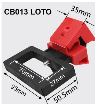
CB013(X) 959433(X) Clamp-on Circuit Breaker Lockout Large Toggle Up to 70mm. Toggle width 18, 32, 42, 70mm.
