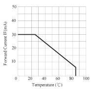
FORWARD CURRENT VS. AMBIENT TEMPERATURE
