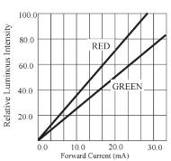
FORWARD CURRENT VS. LUMINOUS INTENSITY
