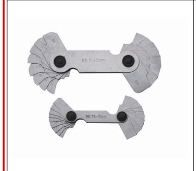
Penknife style Radius Gauges have accurately machined blades which are suitable for checking both internal and external radii. Each blade is marked with its size
