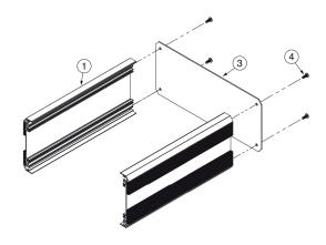
1. Install ③ front/rear panel to ① side frame and secure with ④ Umbrella Phillips Screw M5-10 (Dog Point).
