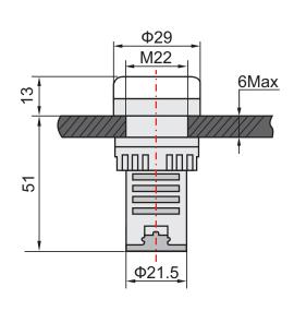
RS Pro Dual Colour LED Indicators are ideal for providing highly reliable indication with the added benefit of saving space by effectively combining two indicators into one. Fitting in the same 22.5mm cutout this is an easy solution to include extra functionality within existing panels as well as new designs.
