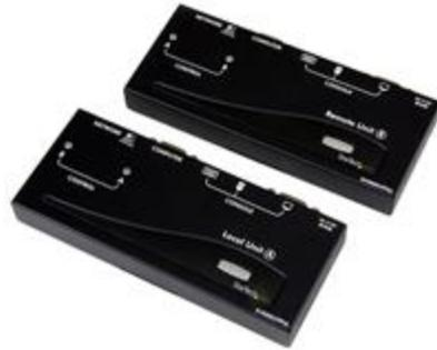
The SV565UTPUL Long Range USB VGA KVM Console Extender over Cat5 UTP (1000 ft) lets you control a server, computer or multiple computers (connected through KVM Switch) over a standard Cat5 or Cat6 UTP network cable connection, at distances of up to 1000ft (300m) away.
