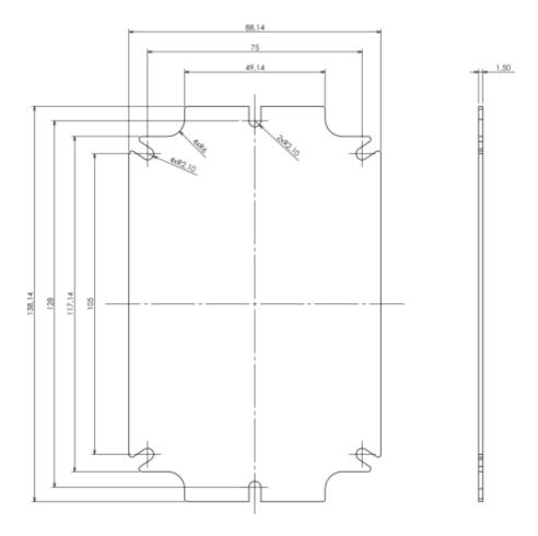
All dimensions are given within +/-0,5mm tolerance
