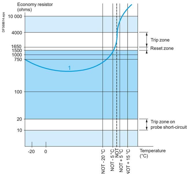
1 3 probes type DA1●●● (250 Ω at 25 °C) in series.
