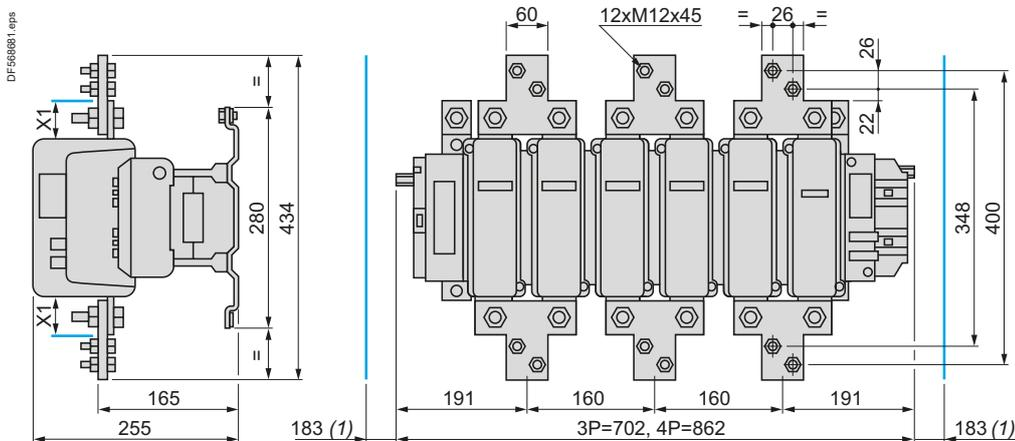
X1 (mm) = Minimum electrical clearance according to operating voltage and breaking capacity.
