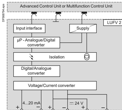
100 Ω < load < 500 Ω ≍ 30 V max and 40 mA min
