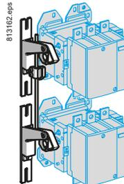
Contactor pairs assembled using 3 contactors of identical or different ratings, type :
