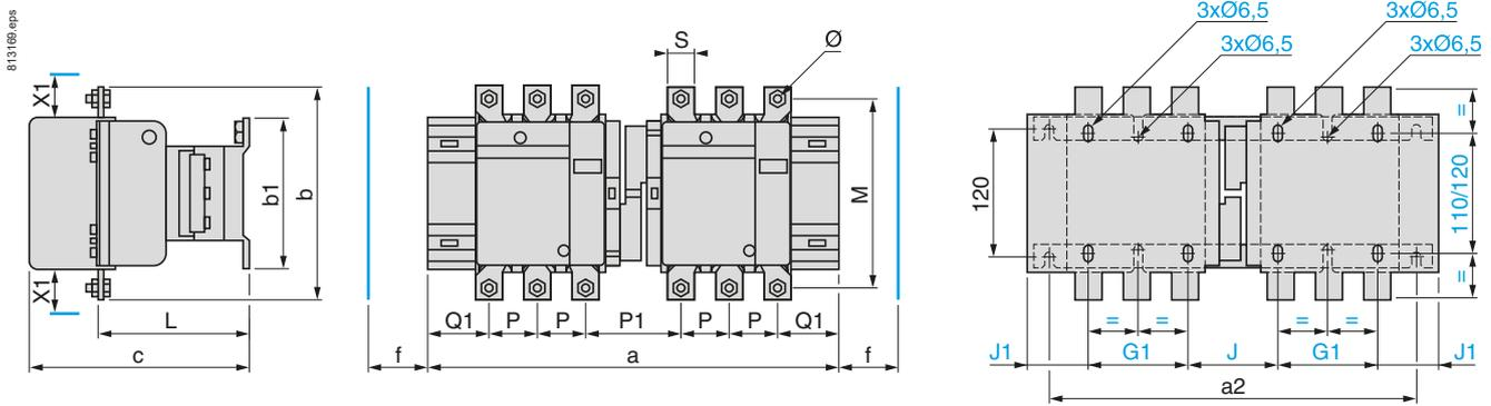
f - Minimum distance required for coil removal.
