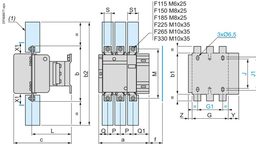
X1 (mm) = Minimum electrical clearance according to operating voltage and breaking capacity.
