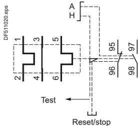
Note: If pre-wiring is not required, break off the 2 links located on the thermal overload relay.
