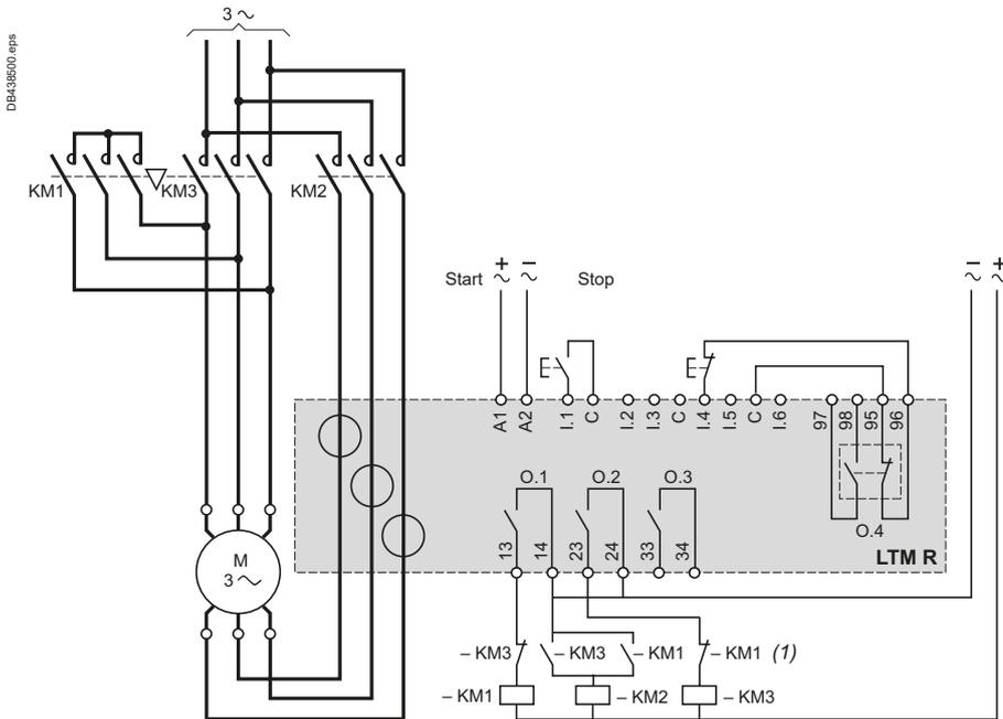
(1) Contacts for interlocking KM1 and KM2 are not obligatory because the controller electronically interlocks outputs O.1 and O.2.
