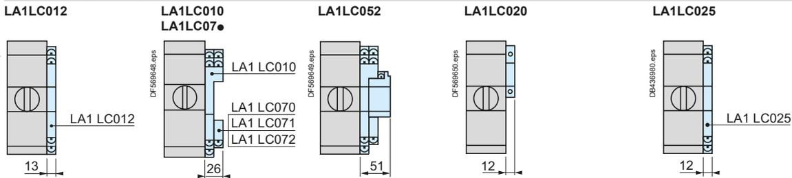
For mounting on reversing Integral motor starters
