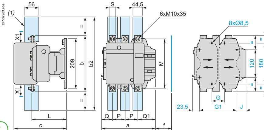
X1 (mm) = Minimum electrical clearance according to operating voltage and breaking capacity.
