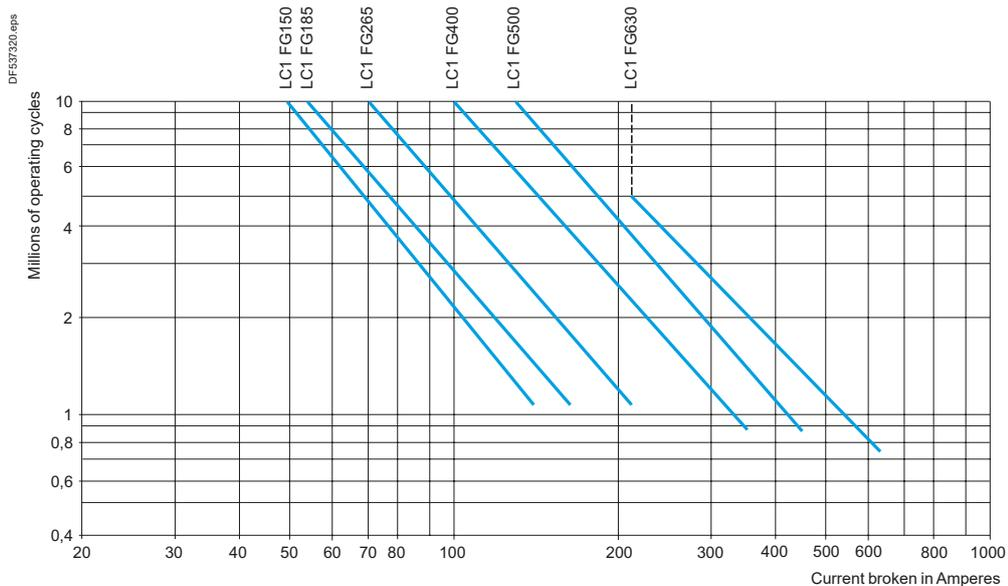
Control of 3-phase asynchronous squirrel cage motors with breaking whilst running. The current broken ( $I_e$ ) in category AC-3 is equal to the rated operational current of the motor.
