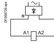
(1) Breaking on ~ side. Drop-out time 50 ms.
