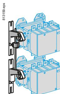
Contactor pairs assembled using 2 contactors of different ratings, type :
