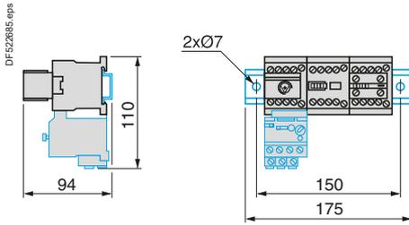
On starters LC3D09A to D18A, a connection block is mounted on the upper part of contactor KM2, increasing the overall height of the product by 6.5 mm.
