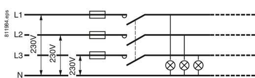
The maximum number of lamps which can be operated per phase is equal to the total number of lamps in the "single-phase 230 V" table.
