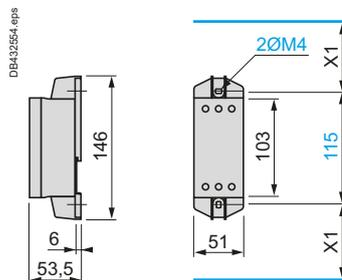
X1: Electrical clearance = 30 mm for  $U_e \leq 690$  V
