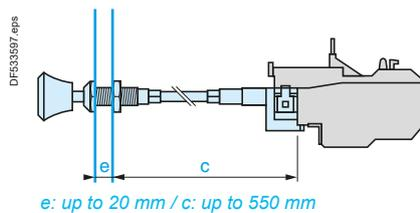
Mounting with cable bent
