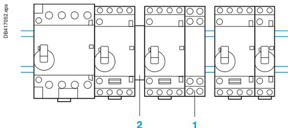
It is advisable to mount electronic units at the bottom of the modular panel and to separate them from electromechanical units by a space equal to one module **3** or by 2 ventilation 1/2 modules GAC5.
