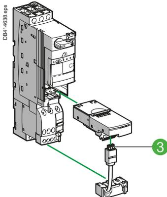
The LULC08 communication module, combined with the power base and control unit is used to control Ultra starters-controllers via CANopen bus. The LULC08 communication module is slave type.
