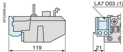
(1) Can be mounted on RH or LH side of relay LRD3..., LR2D35... or LR9D.
