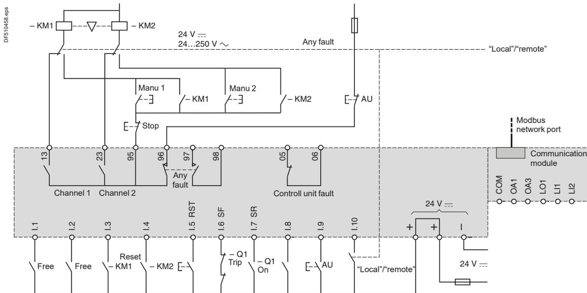
(1) The contacts are represented with controller powered up and not in a fault condition.
