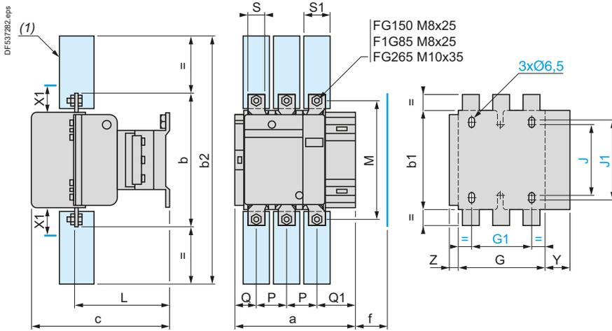
X1 (mm) = Minimum electrical clearance according to operating voltage and breaking capacity.
