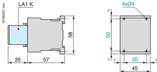
On mounting rail NSYSR200BD or NSYSR200 (≥ 35 mm)
