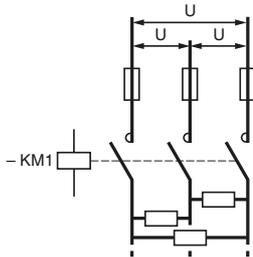
Circuit controlled by 3 poles of the contactor.
