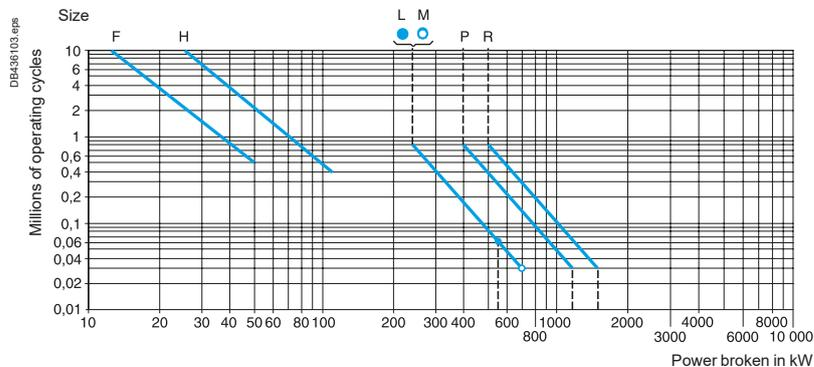
Example: 30 kW motor, 500 V-70 A in category DC-3:  $P \text{ broken} = U_e \times 2.5 I_e = 500 \times 2.5 \times 70 = 86 \text{ kW}$  or 43 kW per pole.
