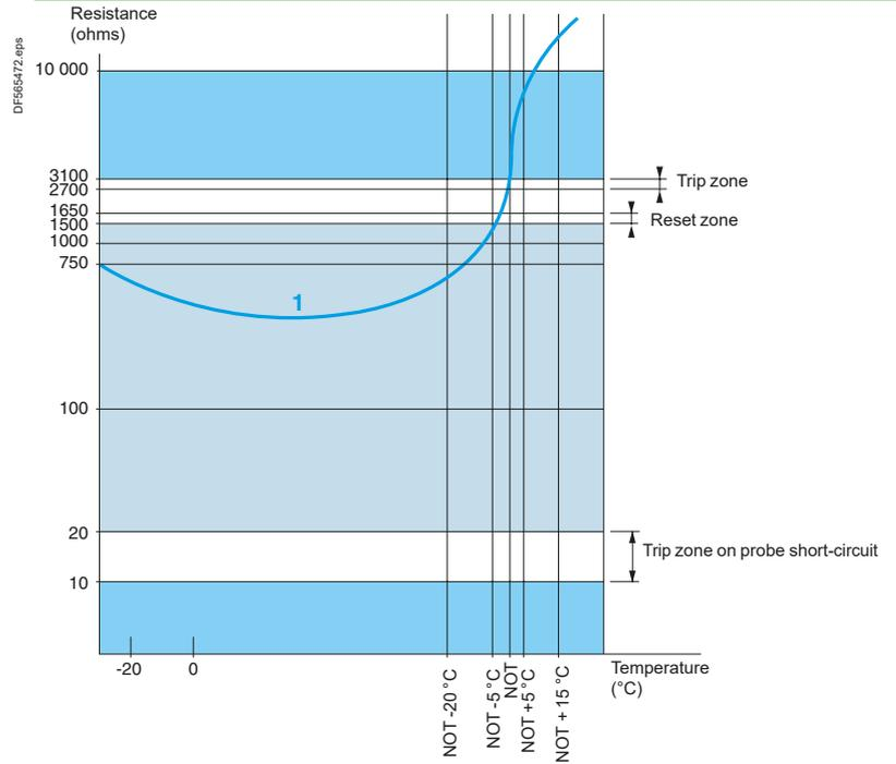
1 3 probes type DA1TT●●● (250 Ω at 25 °C) in series.
