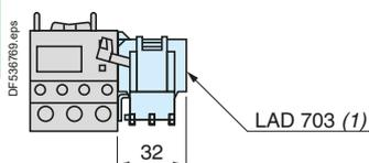
(1) Can only be mounted on RH side of relay LRD01...35 and LRD313...380.
