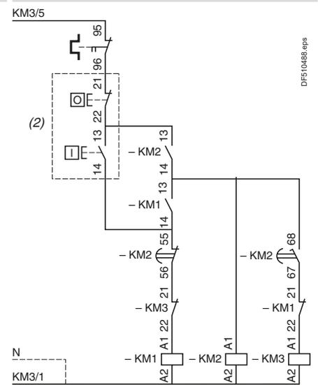
Note: LC3D09A to D18A: Mechanical interlock between KM3 and KM1.
