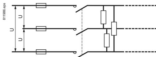
Heating by resistive elements or by infra-red radiators, convectors or radiators, heating ducts, industrial furnaces. The current peak between the hot and cold states must not exceed 2 to 3 I<sub>n</sub> at the moment of switch-on.
