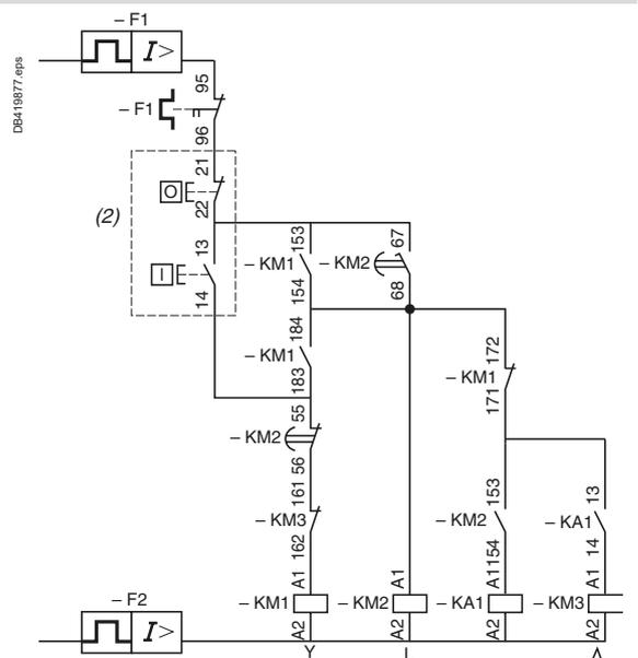
(1) Recommended cabling for reversal of motor rotation (standard motor, viewed from shaft end).
