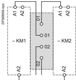
**Mechanical interlock without integral electrical contacts**
