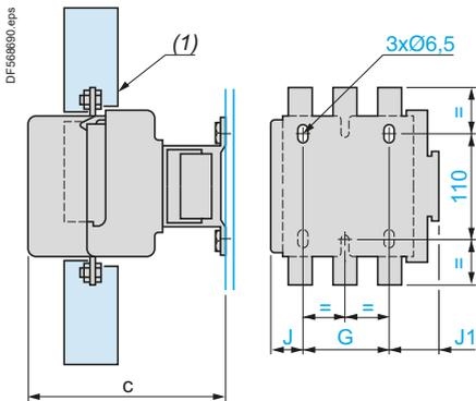
On pre-slotted mounting plate AM1PA, PB, PC
