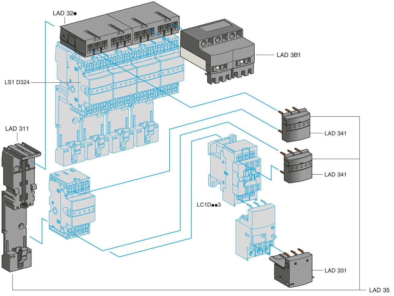
Power circuit pre-wiring components
