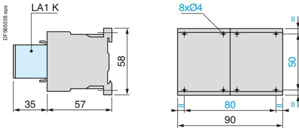
On mounting rail NSYSR200BD or NSYSR200 (≥ 35 mm)
