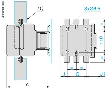
On pre-slotted mounting plate AM1PA, PB, PC
