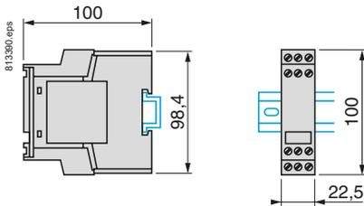
Mounting on 1 L rail (with adapter RHZ 66)
