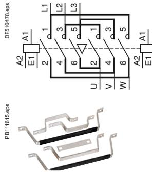
3 or 4-pole changeover contactor pairs
