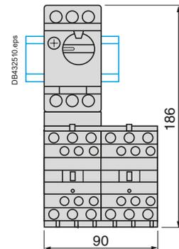
LC1D, LC2D contactor with AC or DC coil on mounting rail
