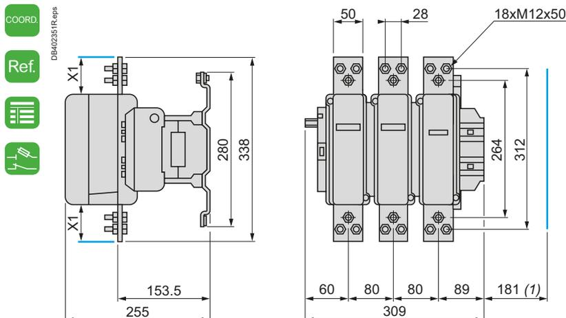
(1) Minimum distance required for coil removal.
