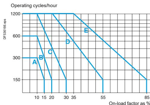
For an on-load factor of 17 % at 180 operating cycles per hour, the above curve indicates zone B. If the maximum current broken is 200 A, the table above will lead to the selection of a size H contactor. Referring to the electrical durability curves, it can be seen that the contactor will have a life of 1 million operating cycles. Where a higher value of electrical durability is required, 2 million operating cycles for example, size K would be recommended.
