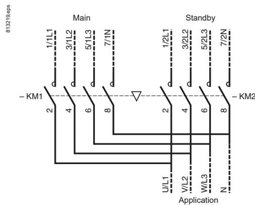
The 2 contactors must be mechanically and electrically interlocked to prevent any paralleling, even transitory, of the two supplies.
