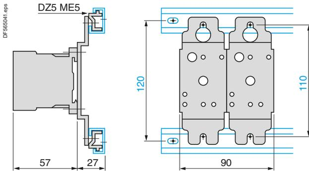
On printed circuit board for reversing contactors or 2 contactors mounted side by side.
