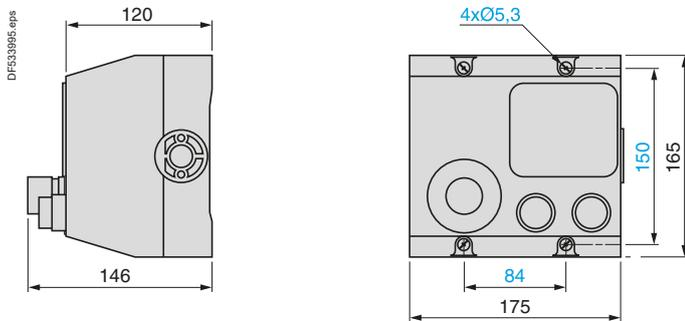
Cut-outs or blanking plugs for cable glands at the top and at the bottom 2 x 13 P and 2 x 16 P.
