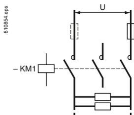
Circuit controlled by 2 poles of the contactor.
