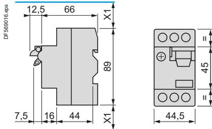
X1: Electrical clearance = 40 mm for  $U_e < 690$  V
