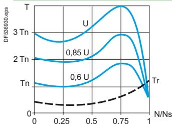
The diagram opposite shows the torque/speed characteristic of a cage motor in relation to the supply voltage. The torque varies in line with the square of the voltage at a fixed frequency. The gradual increase in the voltage prevents the instantaneous current peak on power-up.
