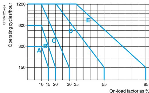
For an on-load factor of 10 % at 400 operating cycles per hour, the curve on the left indicates zone B. If the current broken is 600 A, the above table leads to selection of an **LC1FG400** contactor. Referring to the electrical durability curves, it can be seen that the contactor will be able to perform 350 000 operating cycles. Where a higher value of electrical durability is required, 1 million operating cycles for example, an **LC1FG630** contactor would be recommended.
