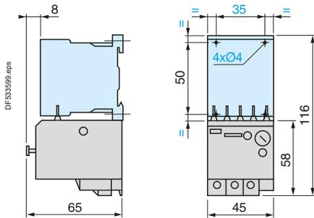
Separate mounting with terminal block LA7 K0064 on 35 mm rail (AM1DP200 or AM1DE200)
