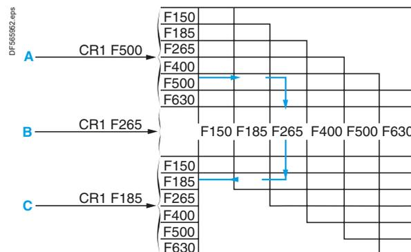
**Warning:** the contactor ratings must be in decreasing size from top to bottom.
