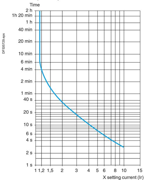
Balanced operation with 2 phases only, from cold state
