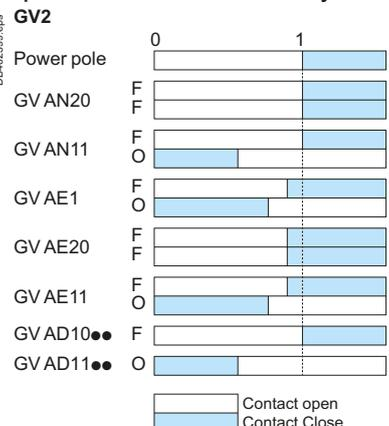
(1) For application example of fault signalling contact and short-circuit signalling contact.
