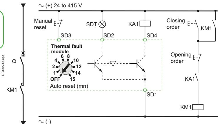
**SD1, SD3:** thermal fault module input power supply
