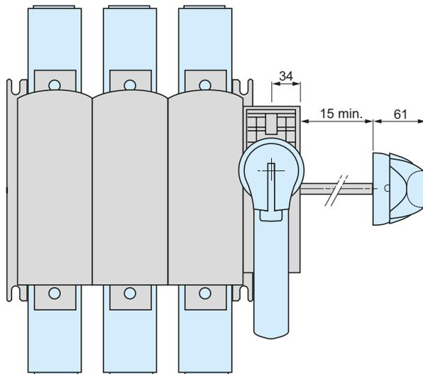
Handle GS2AH570 or GS2AH580 for GS2V and GS2VB (external front-mounted operator)
