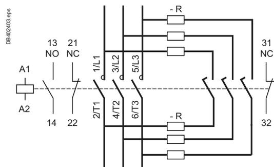
R = Pre-wired resistor connections.
