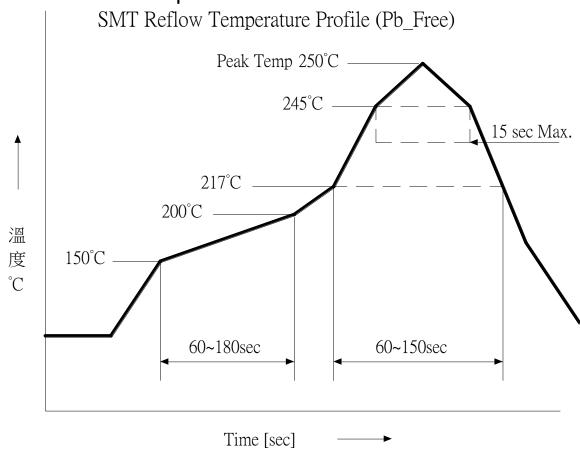
Note: 245℃ is Less than 15 sec. ,but only pass the lead free reflow once.
