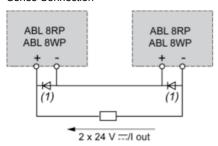
(1) Two Shottky diodes Imin = power supply In and Vmin = 50 V Parallel Connection
