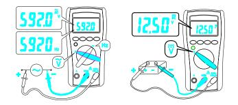
The non-zero display reading is normal when the meter test leads are open, but this will not affect actural measurement accuracy. The meter will show zero or close to zero when the test leads are shorted. In reading AC voltage or current, reading-settling time increases to several seconds at the low end of AC voltage and current ranges in rms models.
