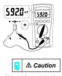
To avoid possible damage to the meter or to the equipment under test, disconnect circuit power and discharge all high-voltage capacitors before measuring capacitance. Use the DC voltage function to confirm that the capacitor is discharged.
