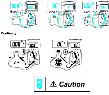
For in-circuit test, turn circuit power off and discharge all high-voltage capacitors through an appropriate resistance load.
