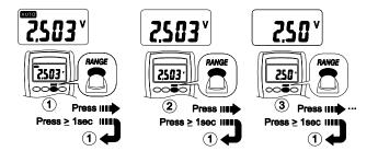
Note - The Range button is pressed to select manual ranging and to change ranges. When the Range button is pressed once, the  $\boxed{AUTO}$  indicator turns off. Press the Range button to select the appropriate range for the measurement you want to make. Press the Range button and hold for 1 second to return to Autorange mode.
