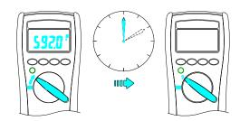
**Note** – If the meter idles for more than 10 minutes, the meter automatically turns the power off. When this happens, the LCD displaying-state of the meter is saved. The meter can be turned back on by pushing any button, the LCD displays the saved state. Pushing *Hold* button to disables the hold state. Any button press or rotary switch change resets the time of Auto Power-OFF.
