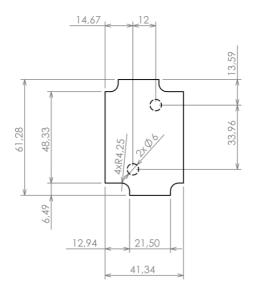
Dashed line shows outline of the mounting boss under PCB board Recommended mounting holes diameter ø3,5mm
