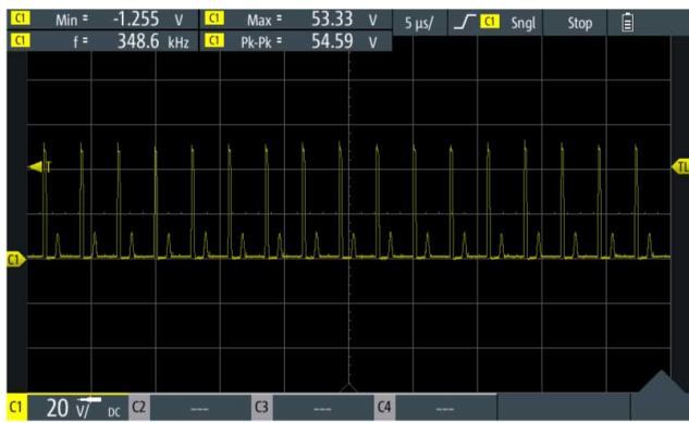
Figure 13. Boost Pulses at MOSFET Q2 Drain Terminal at 5 μs
