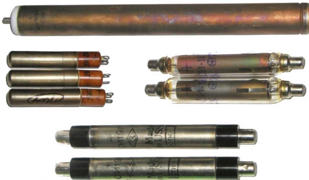
Figure 2. Geiger-Muller Sensor Tubes
