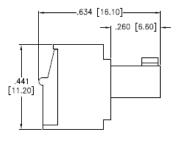
Positions: 02 thru 24 A = .150 [3.81] x No. of Spaces + .181 [4.60] B = .150 [3.81] x No. of Spaces
