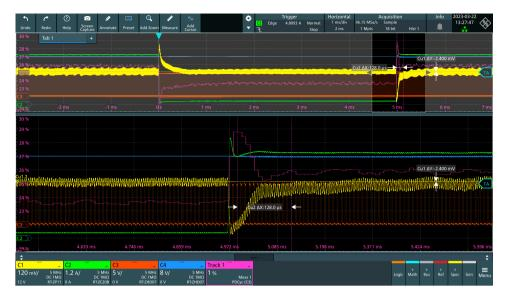
Reviewing control theory shows the 2% deviation comes from higher conduction losses caused by higher output current. The higher losses are mainly generated in the transformer and output rectifier. The additional losses need to be equalized by increasing the positive duty cycle and the track function allows this complex measurement task to be performed.
