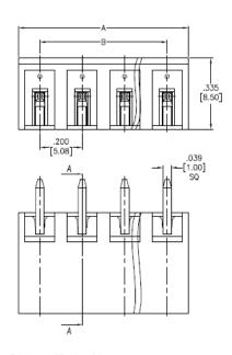
Positions: 02 thru 24 A = .200 [5.08] x No. of Positions B = .200 [5.08] x No. of Spaces
