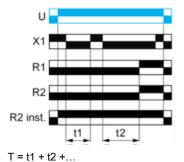
Function: 1 Output with Retrigger / Restart Control
