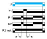
Function C: Off-Delay Relay with Control Signal
