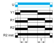
Function Act: On-Delay & Off-Delay with Control Signal & With Pause / Summation Control
