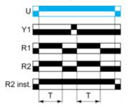
Function W: Interval Relay with Control Signal Off
